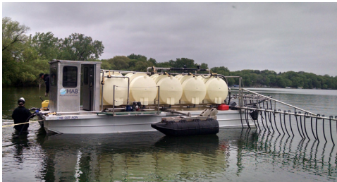
Alum treatment equipment on Lake Riley in Eden Prairie
