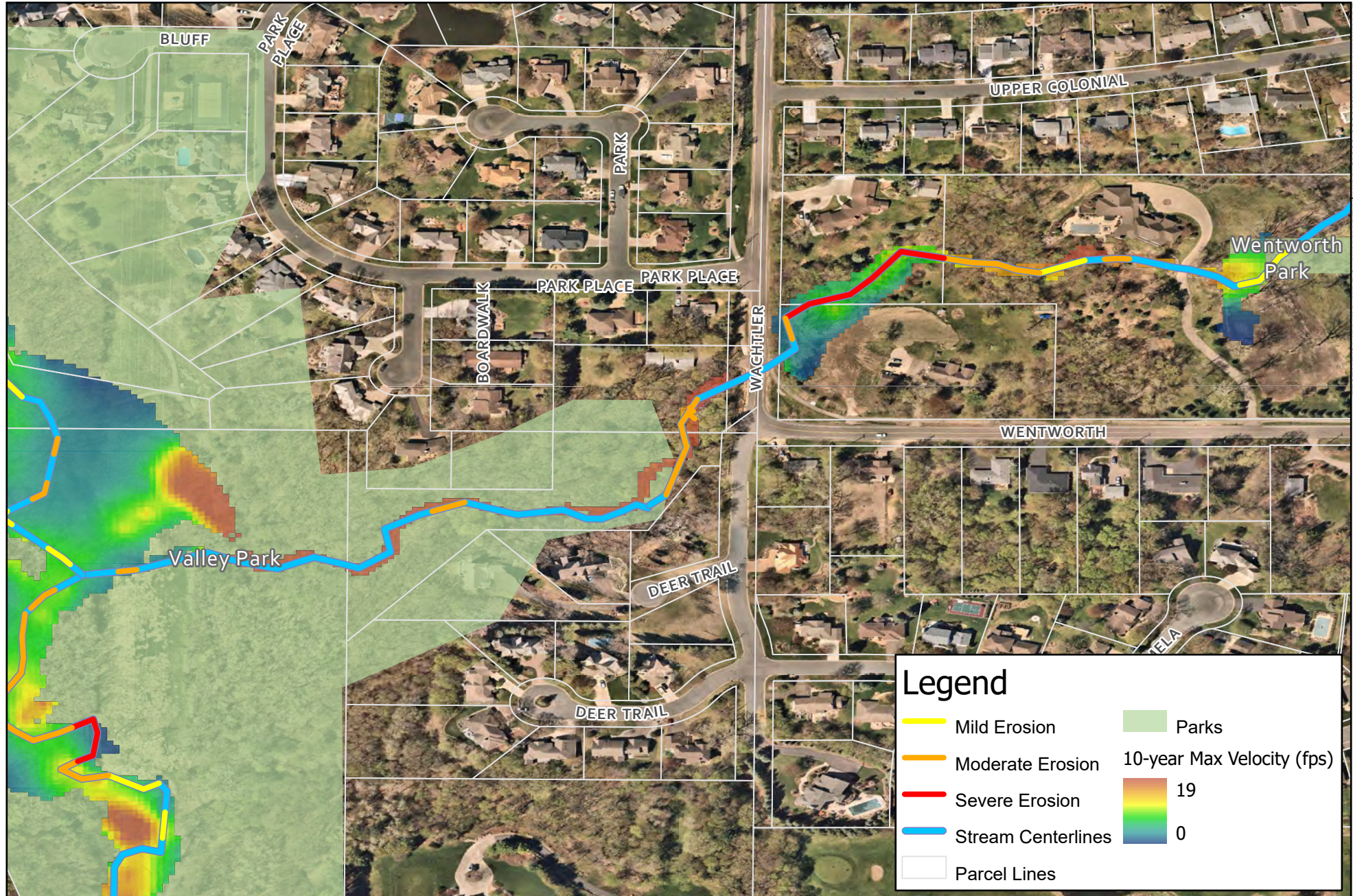
Figure AE.5, 10 Year Max Velocities, Lower and Middle Wentworth Creek Interstate Valley Creek Study Lower Mississippi River Watershed Management Organization
