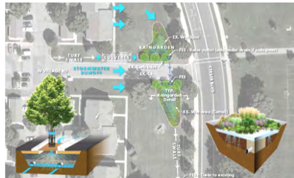
Barr developed this rendering of a potential rain garden BMP in the downtown Chanhassen area to support stakeholder outreach to residents and
