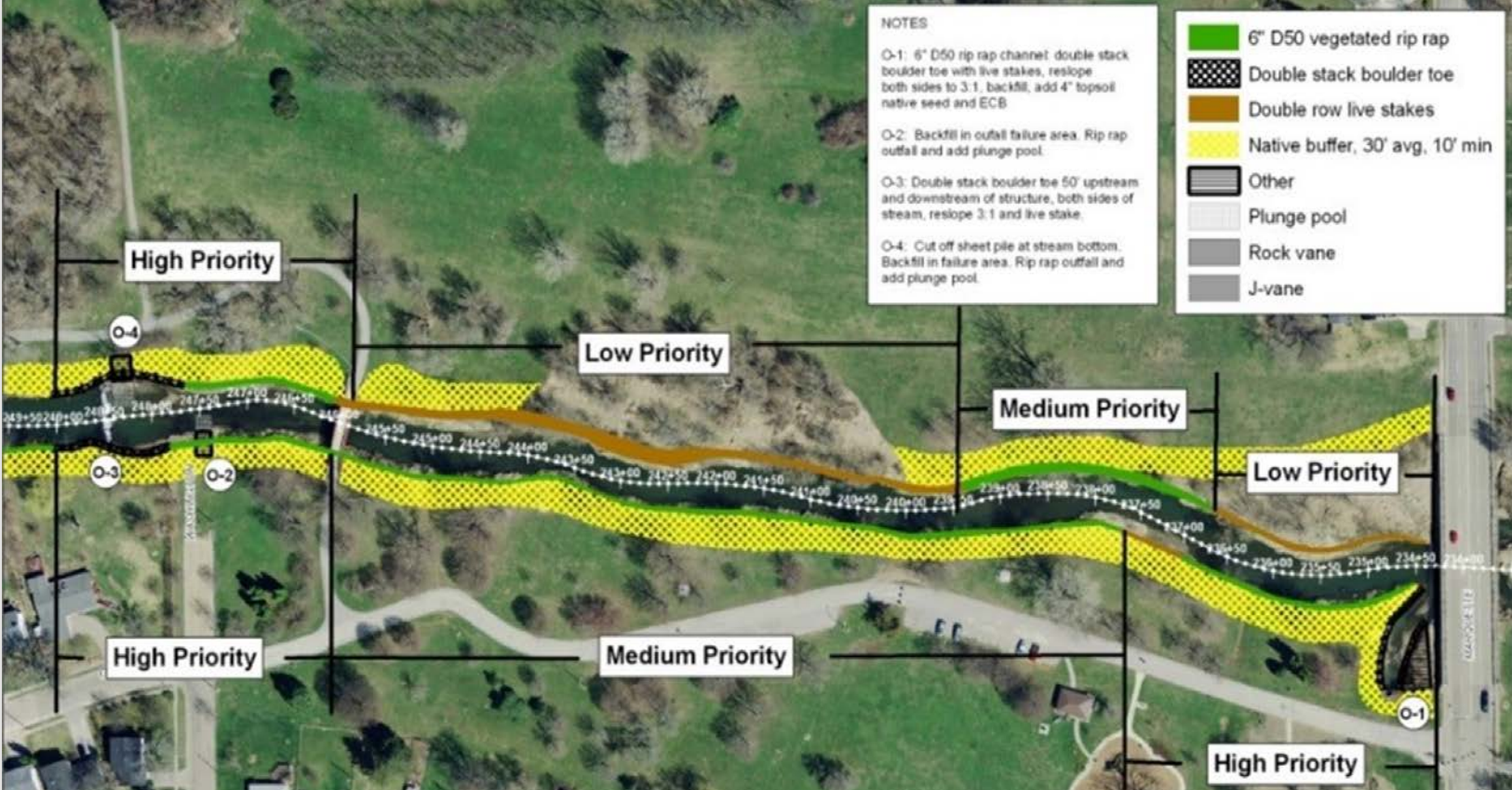
↑ A reach improvement schematic for a subreach of Duck Creek in Davenport, Iowa.
