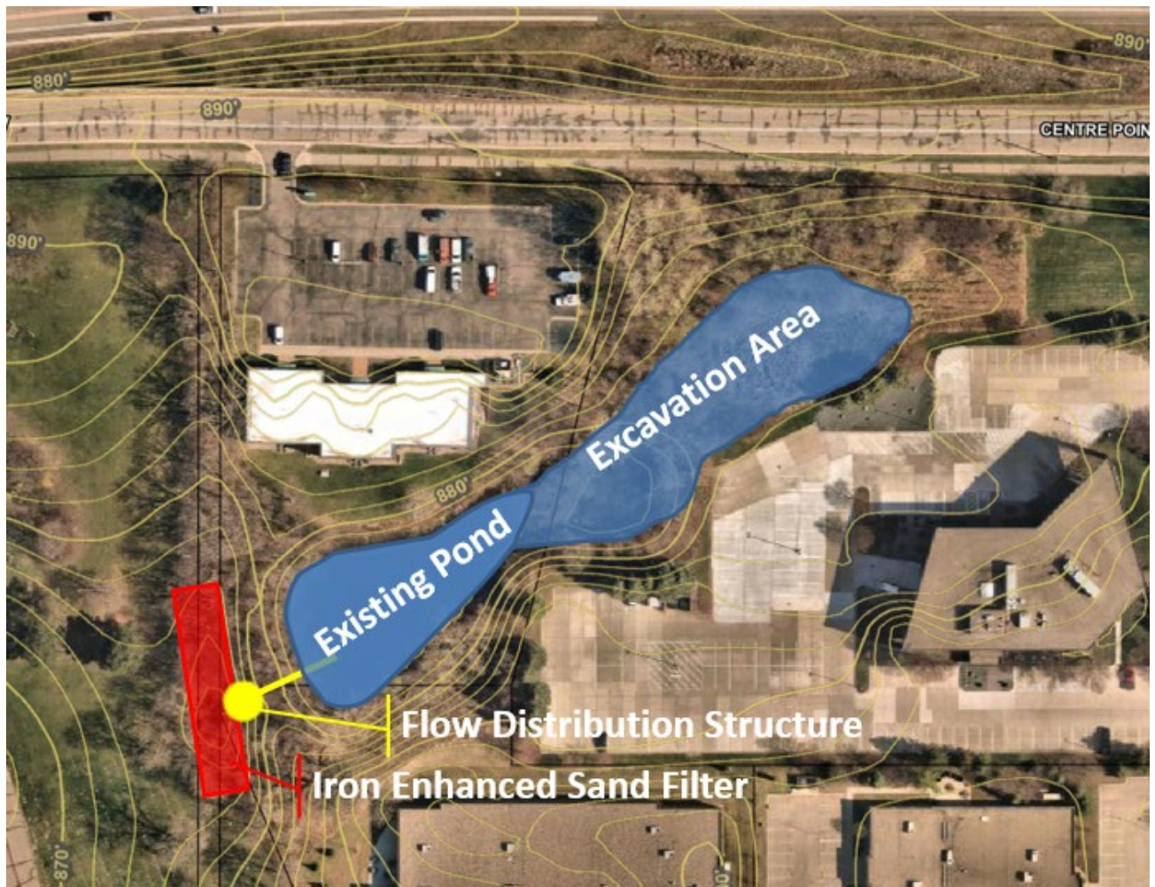
Figure 5-4 Conceptual Design of Stormwater Pond 2 Enhancements
