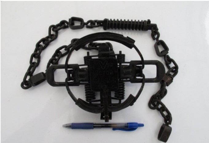
Figure 7. No. 3 padded-jaw foothold trap. All 4 springs should be removed and replaced with 2 springs suitable for a No. 1.5 paddle-jaw foothold.
