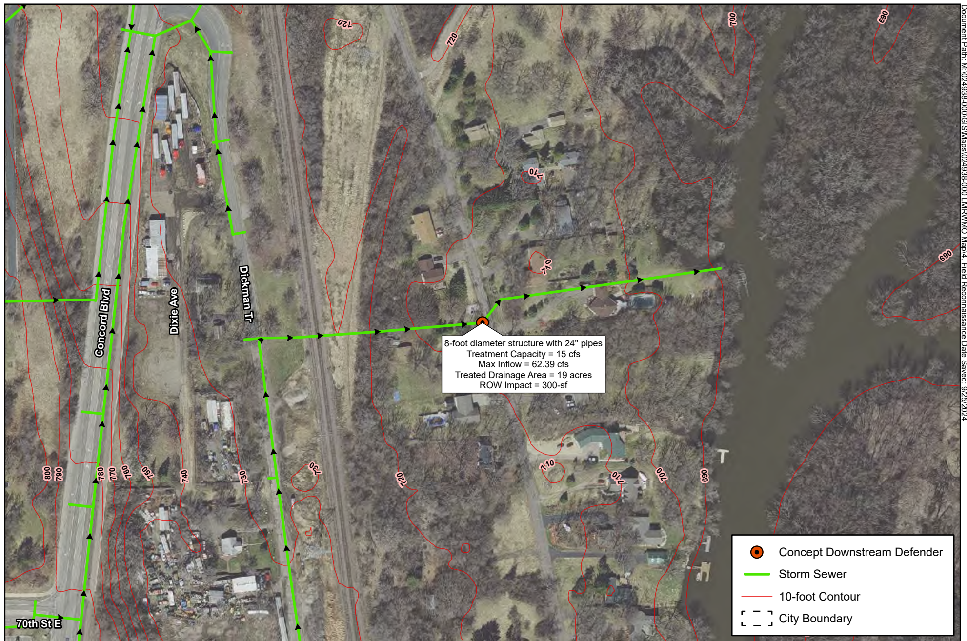
Figure 4.6.7 - IGH Structural BMPs (North)
