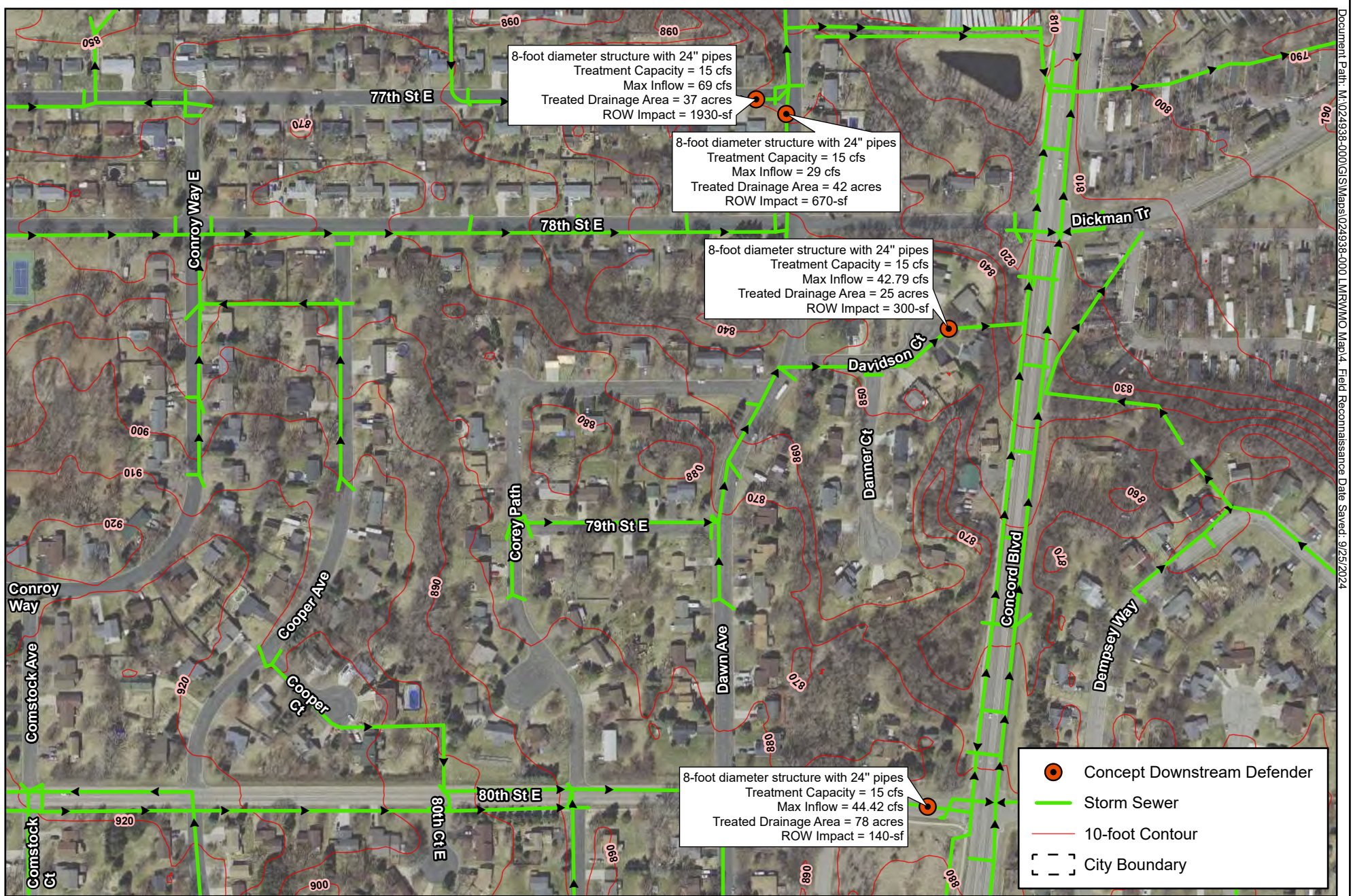
Figure 4.6.8 - IGH Structural BMPs (South)
