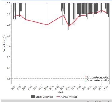
A black and white secchi disc is lowered into the water until no longer visible and measures water clarity. High secchi disc depths indicate good water quality. MPCA standard is 1.4 m (dashed line).
